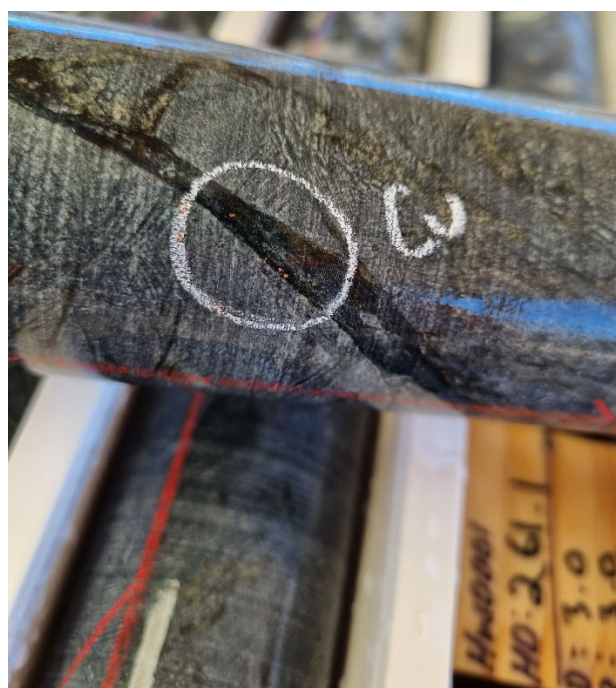
Figures 3 & 4 – Native copper in chlorite-rich veinlets (NQ diamond core) at 255m and 260m.
