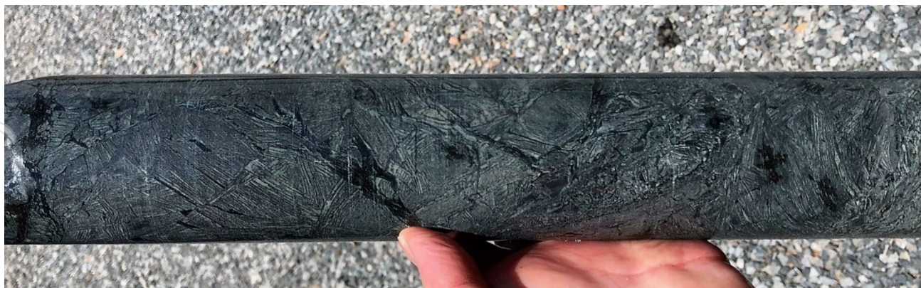
Figure 2 – Spinifex textured komatiite (HQ core) indicating proximity to the top of an ultramafic lava flow, assisting in identifying the number of flows intersected downhole.
